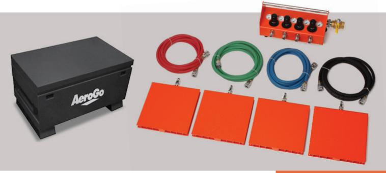
Compact and flexible, the AeroGo® Air Caster Rigging Kit includes all the components necessary to move loads up to 64,000 lbs. depending on module size selected (see back for specifications). The Rigging Kit uses Aero-Casters and compressed air to float heavy loads on a near-frictionless film of air. The kit includes hoses, load modules, a control console, fittings, and aluminum tape. System integrity is protected via a lockable industrial grade storage box for portability and safe storage.
