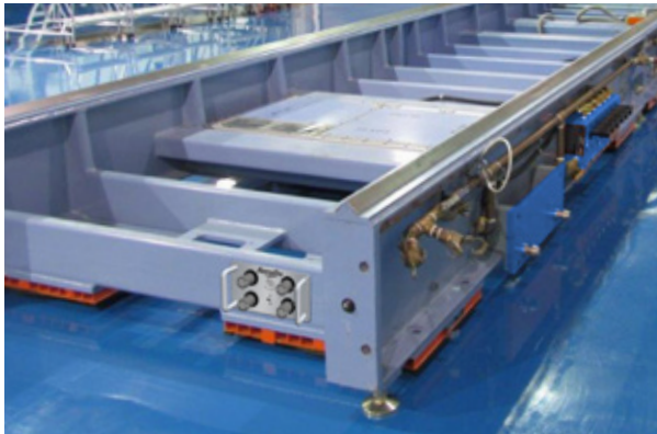
Adding air caster capability makes OEM machinery, tooling and equipment infinitely more mobile and flexible
