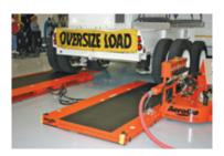
Eliminate Floor Damage. Aero-Planks utilize air casters, which distribute the load weight over a larger surface area than with rollers or wheels. Load stress is spread evenly across the surface, eliminating potential floor damage.
