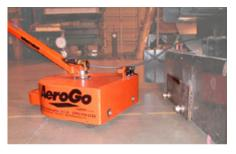
Drive. This allows the drive to be removed or connected to multiple loads or attachment locations. A drive would normally be designed for attachment to a structure that includes a Guide Wheel for car-like steering. Two drives may be connected to a structure on each end for greater omni-directional steering options or more precise positioning.
