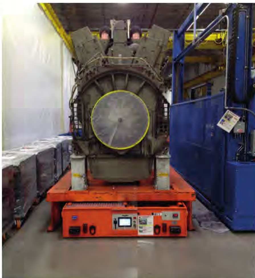
Easily placed under a CNC machine, air casters then float the weight of the load, eliminating the potential for floor damage.
