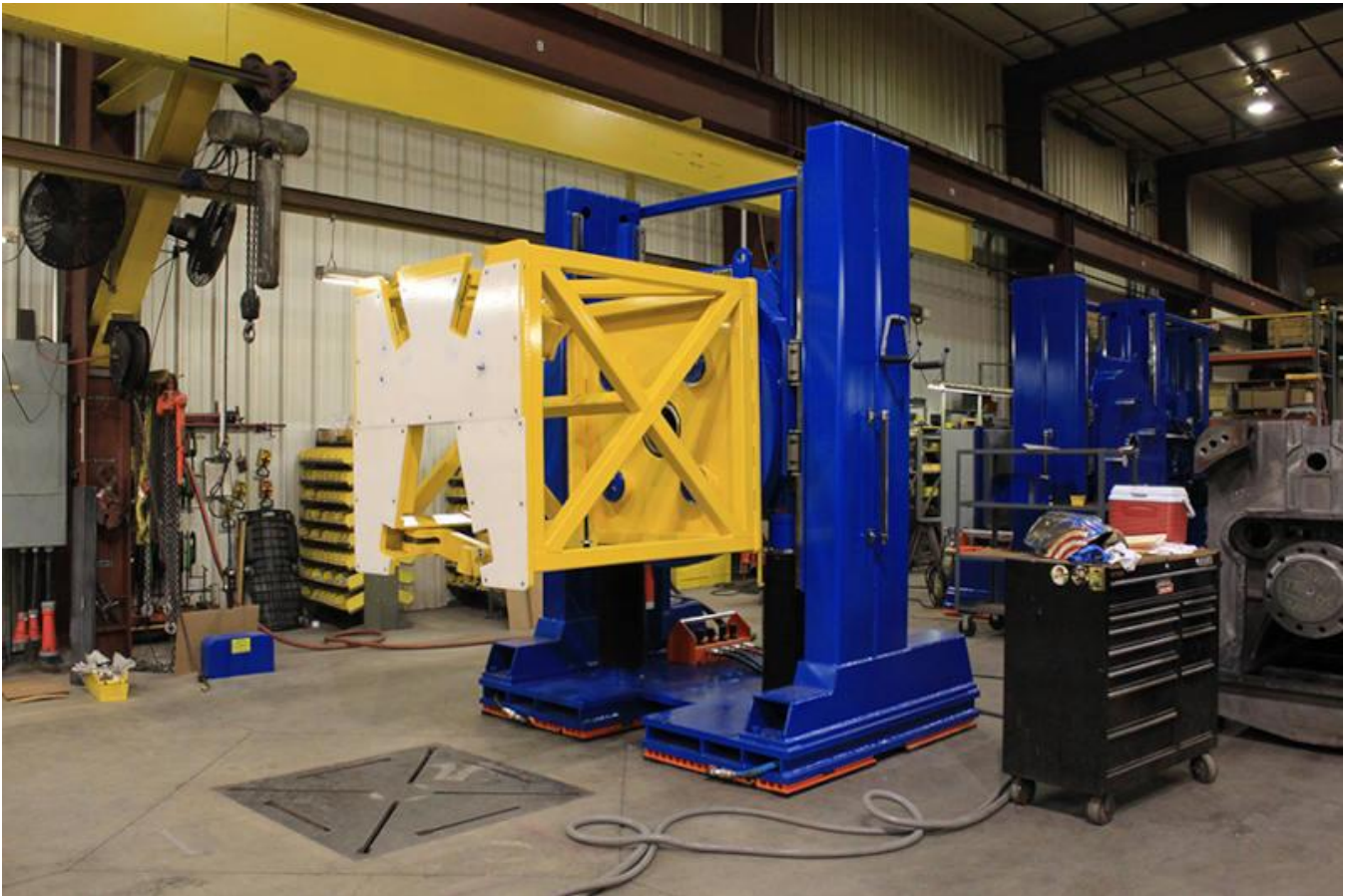
Short moves in a flexible assembly line benefit from an untethered load movement option, such as an air cushion vehicle. Courtesy: AeroGo
