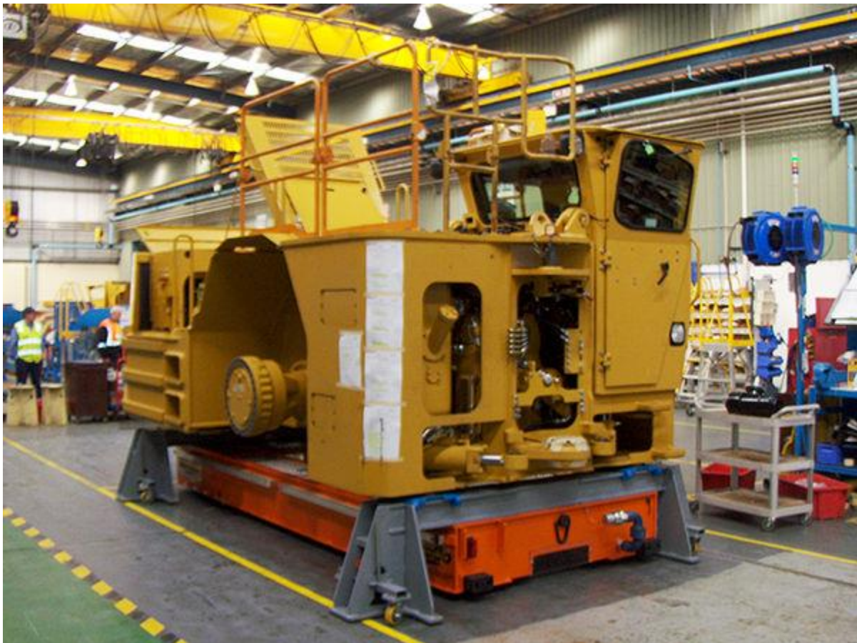
Two material handling options work in tandem here: an embedded air caster system moves a rebuild engine positioner below a crane. Courtesy: AeroGo
