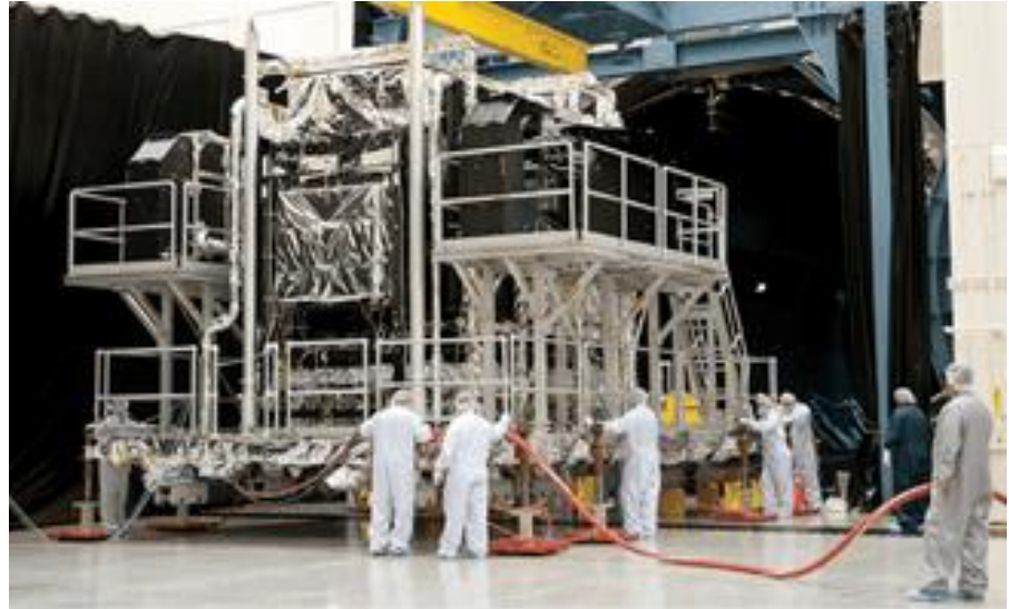
Smooth, vibrationless, and precise movement provided by air casters makes it possible to move satellites into constrained areas where cranes cannot reach. Photo credit: Lockheed Martin
