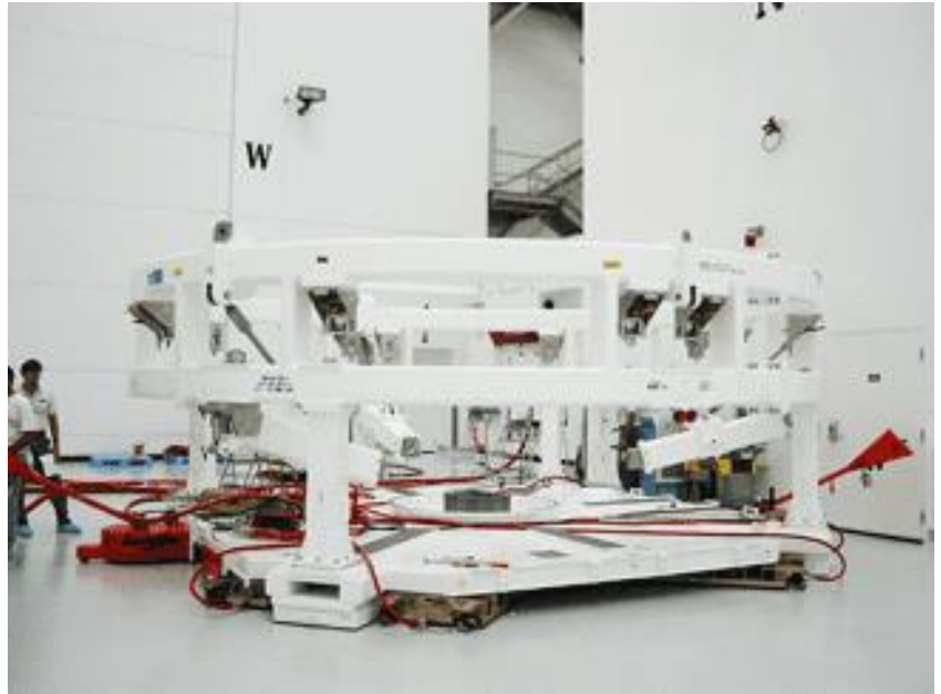
Two operators can float this cleanroom turntable into position. Photo credit: AeroGo
