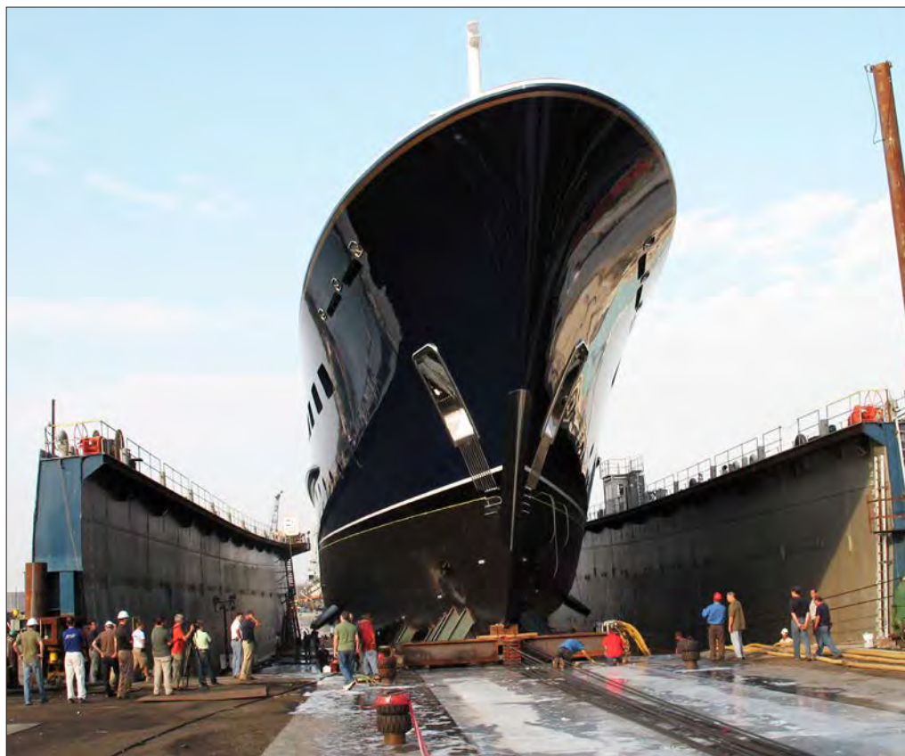
2998 Ton Yacht Moved on Air Bearings in a Shipyard.
