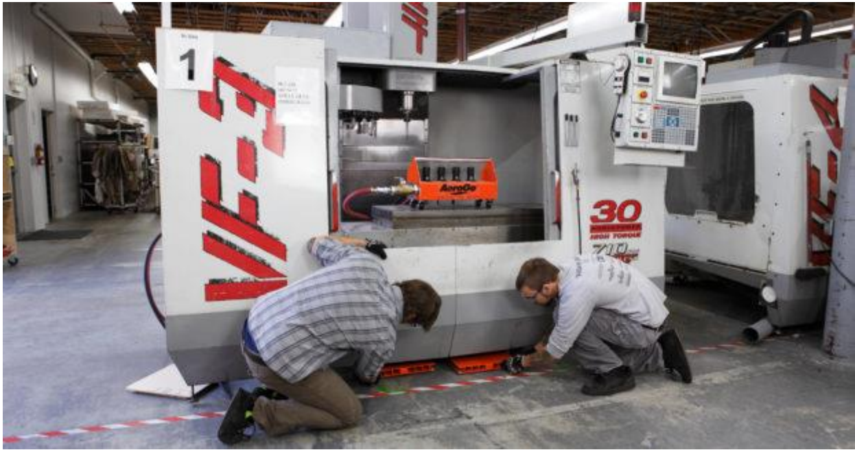
Operators place air casters under a CNC machine to move it into a sequential position in the work flow.
