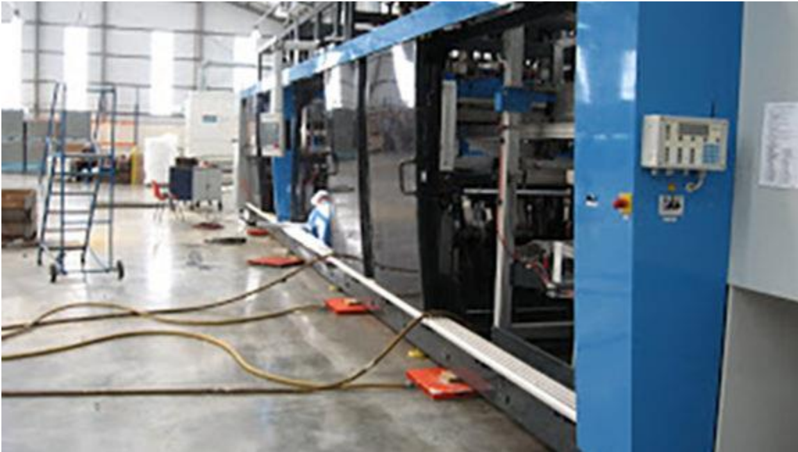
Air casters fit within the footprint of the machine, minimizing the maneuverable space required.
