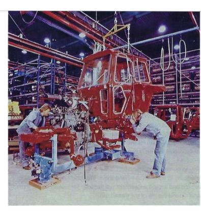
are precisely joined in a process called equipment mating. With traditional crane use, major components are suspended and lowered to line up one component with another. Both components could be the size of houses and weigh as much as 50,000 lbs. There is an element of danger here because workers have to position themselves between and under multi-ton steel parts to move suspended components into place to mate the sub-assemblies.
