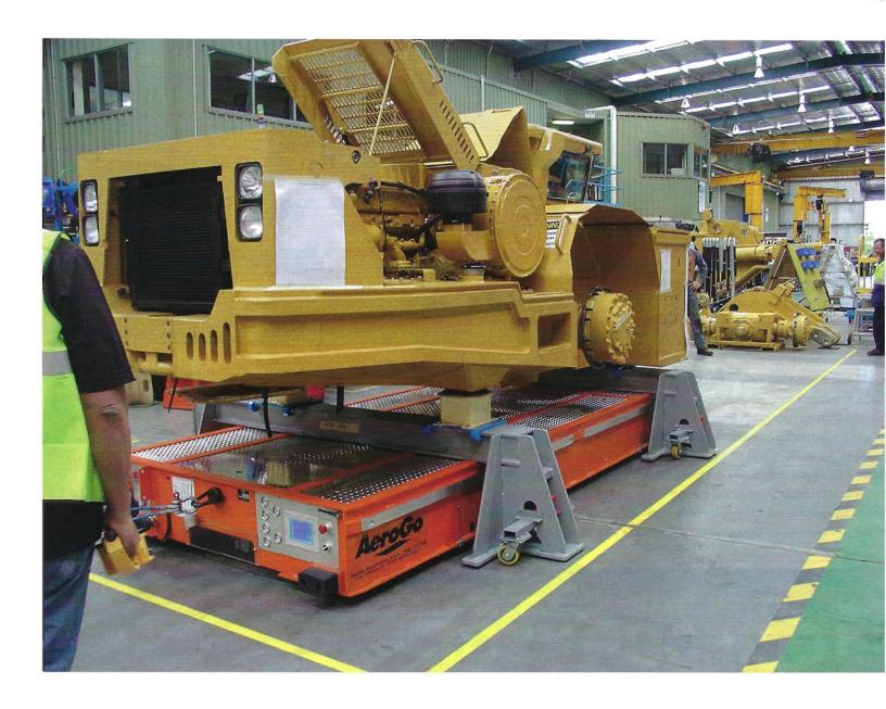
depending on the needs of the manufacturing process. In the tractor-building process, a small team of operators is all that is needed to guide the air transporter into position.
