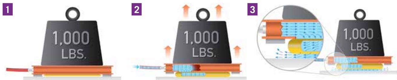
1. The red air hose feeds into a base module (orange) with an air caster (yellow) underneath. 2. Compressed air inflates the air caster and creates lift. 3. Excess air escapes the air caster, creating a film of air that floats the load like an air hockey puck.
