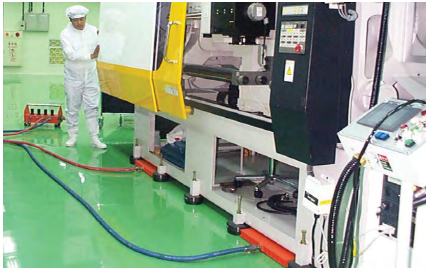
Figure 4. Heavy machines floating on air casters do not pose any risk of damaging epoxy floors.
