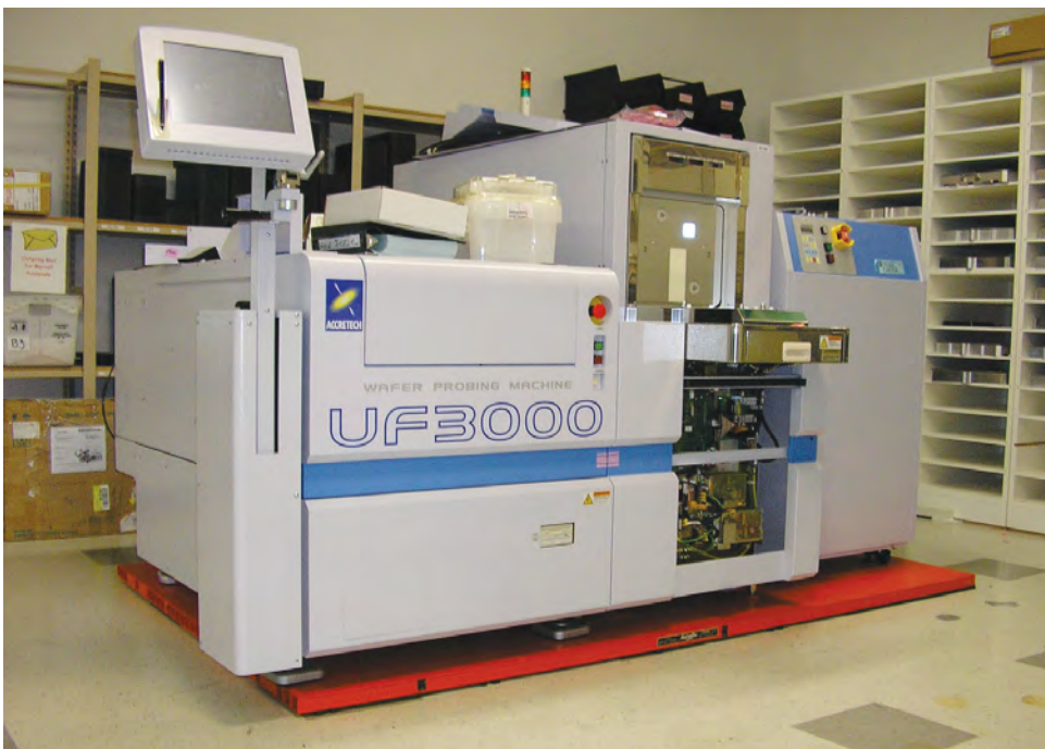
Figure 1. A 4800 lb. test cell wafer prober is moved 30-40 feet, four times a day, on an air caster pallet over VCT flooring.
