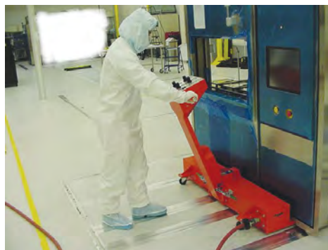
Figure 3. It only takes 5-25 pounds of force for a single operator to move up to 5,000 lbs. on air casters.
