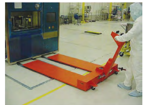
Figure 3. It only takes 5-25 pounds of force for a single operator to move up to 5,000 lbs. on air casters.
