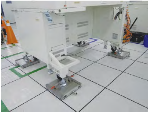
Figure 2. With the machine's wheel placed on the aluminum square housing the air caster, weight is efficiently redistributed, alleviating any issue with floor point loads on raised floors.
