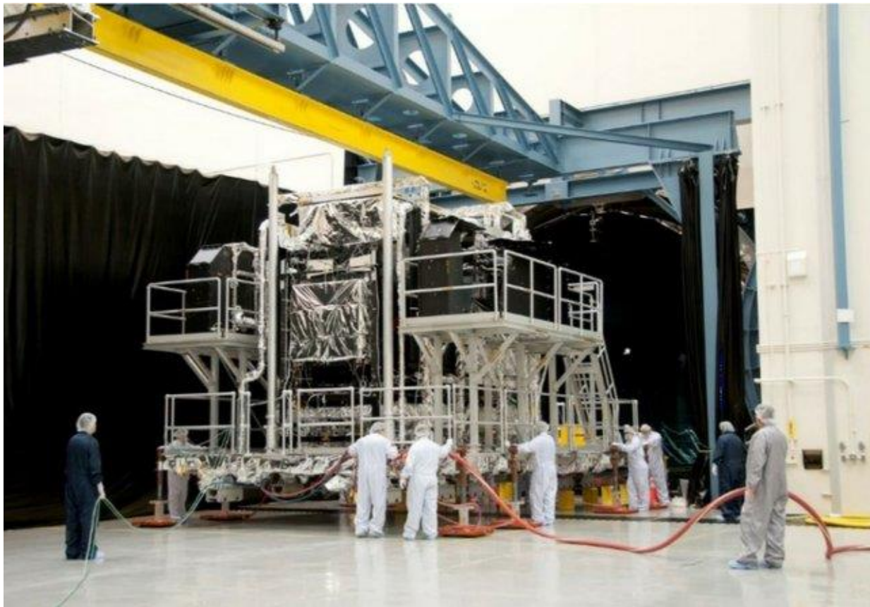
SBIRS 10, 656 lb. satellite moving into test bay on air casters. Source: AeroGo
