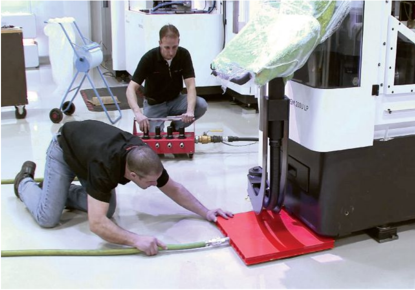
The air caster system slides under the equipment to be moved, fitting neatly within the footprint of the machine.
