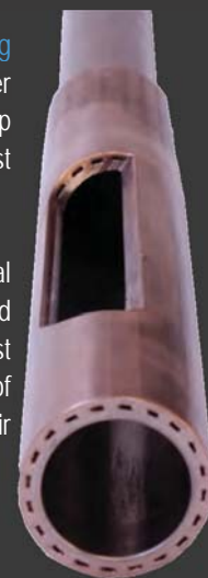
Intentional Leak Path Created Between Internal & Outer Tube
