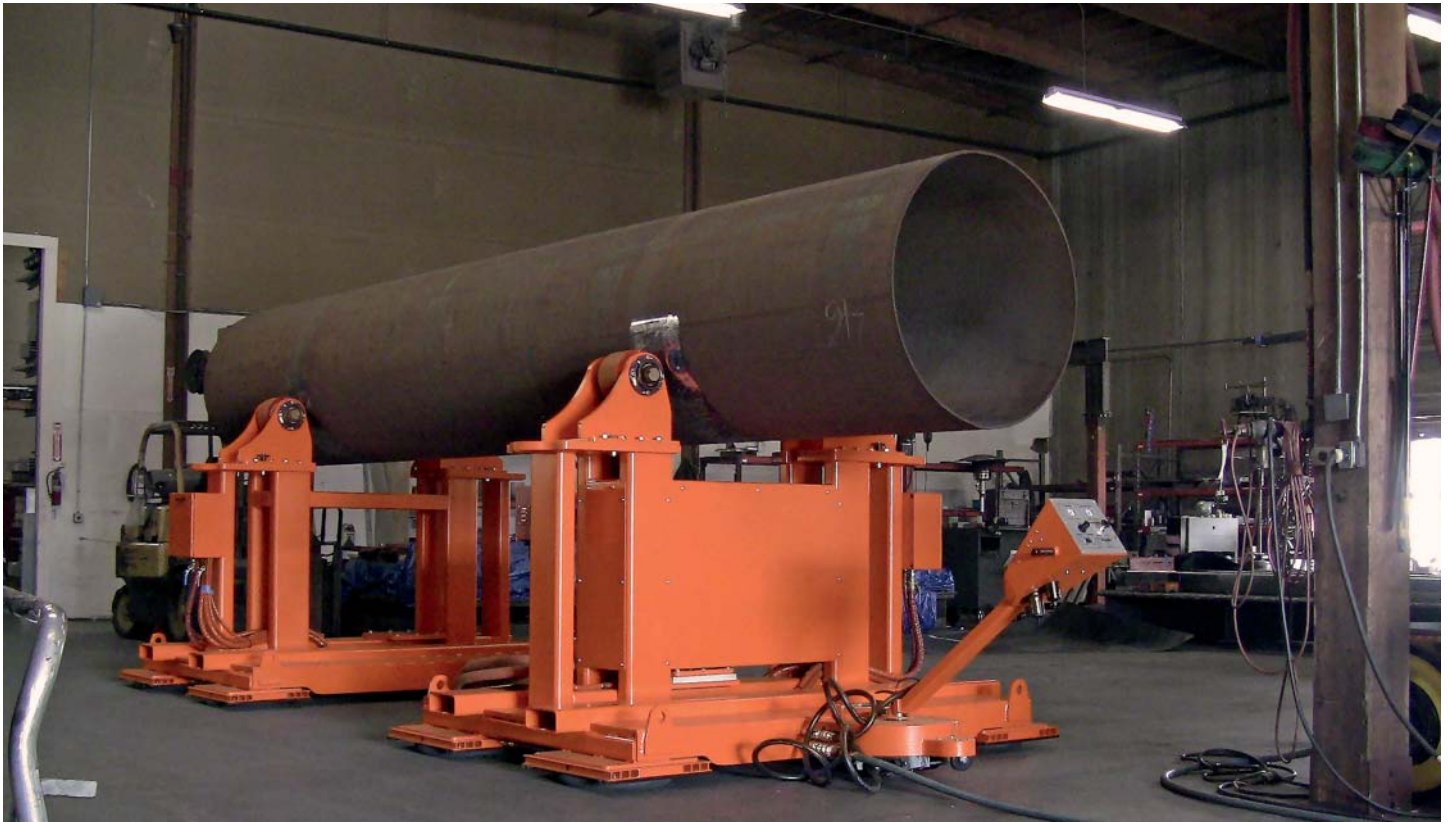
➤ An air caster vehicle featuring a synchronous guide wheel mechanism to rotate a 40' cylinder used to build larger heat exchangers, boilers and chillers.
