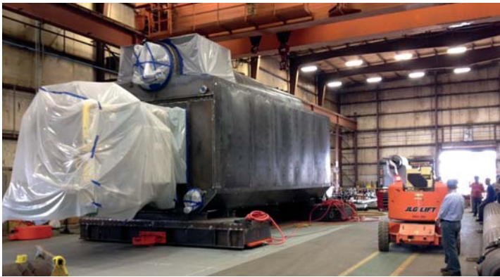
➤ 100 ton boiler floats on air casters. Two operators use power drives to control the move through the plant.
