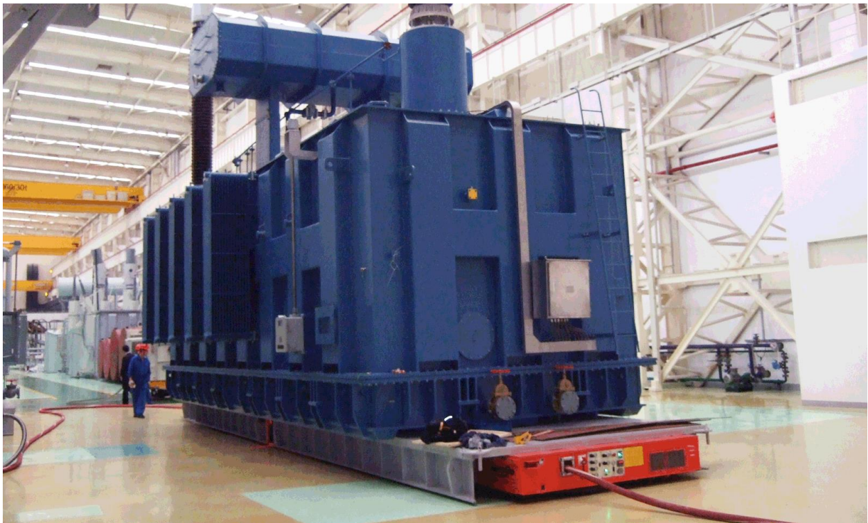
Tandem air cushion vehicles transport transformers up to 800 tons.
