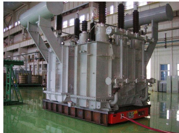
A single air cushion vehicle floats up to 400 tons.
