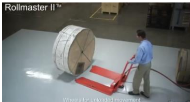
Slide the Rollmaster™ under the roll
