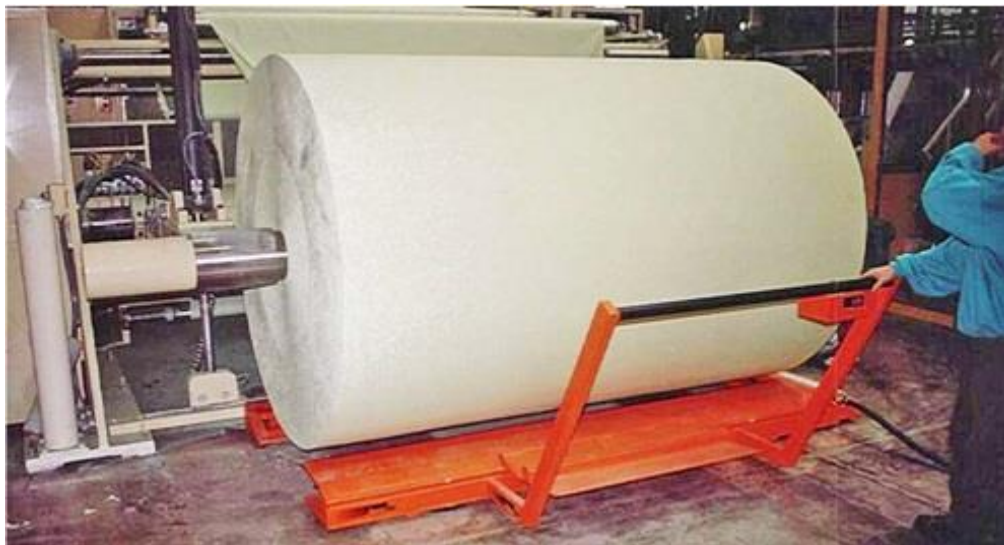
Purpose-built roll handler positions the roll on a spindle
