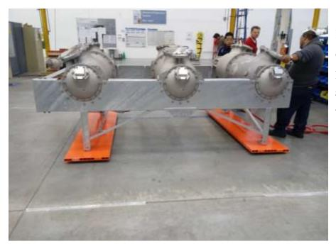
Repositioning components in the production line is safe, simple and quick when they are floating on air.
