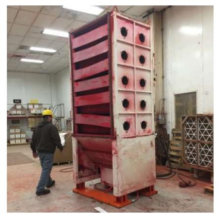
Loads as small as this 2000 lb. powder coating rack are easily moved by a single operator when floating on air bearings.
