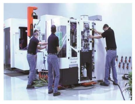
The ability to move 14,000 lb. machines in restrictive areas and eliminate damage to epoxy floors makes air caster rigging systems an attractive alternative to forklifts.
