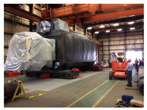
Boilers and pressure vessels up to 100 tons move through a factory on a recurring basis through welding, manufacturing and assembly processes.
