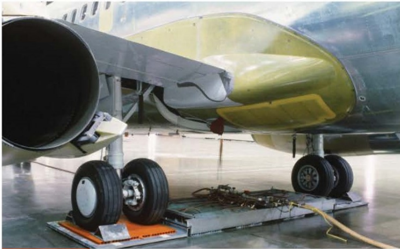
Airplane manufacturing was the first industry to capitalize on air bearings as a flexible and safe load movement method.
