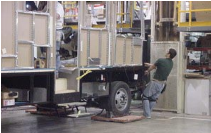
A worker singlehandedly moves a mega RV to a new station in the assembly line.
