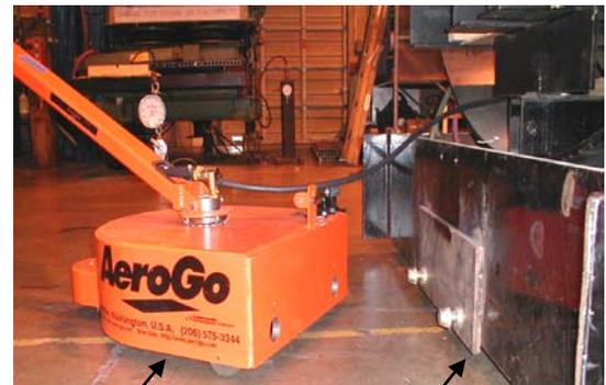
*Aero-Drive positioned to meet Quick Attach plate mounted on load. The detachable Quick Attach “QA” mechanism allows you to utilize one drive for multiple loads, providing exceptional value and flexibility.*
