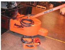
**Optional Guide Wheel Assembly:** (shown unassembled). Attaches to pallet load to provide positive positioning control and prevent potential side drift on slopes. Controls can be added to the drive panel for easy adjustments and operation.
