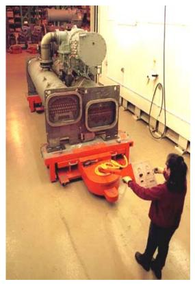
Aero-Drive makes it easy for the operator to steer and control a 20-ton heat exchanger using swing-arm & fingertip controls. (Shown: AG1250E-QA Aero-Drive on a custom engineered Transporter).
