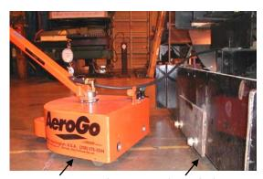
Aero-Drive positioned to meet Quick Attach plate mounted on load. The detachable Quick Attach "QA" mechanism allows you to utilize one drive for multiple loads, providing exceptional value and flexibility.
