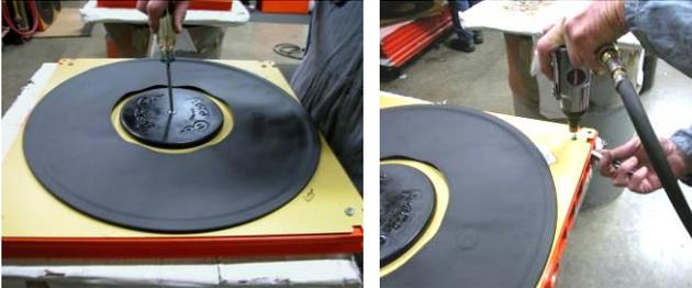
**STEP 2:** Remove the center bolt, center landing pad, and corner mounting bolts. On 27-inch models and larger, corner pads and a center pad are used. (NOTE: For Gapmaster models, no center-landing pad is used. Instead, corner-landing pads are used.) **Be sure to save all hardware.**
