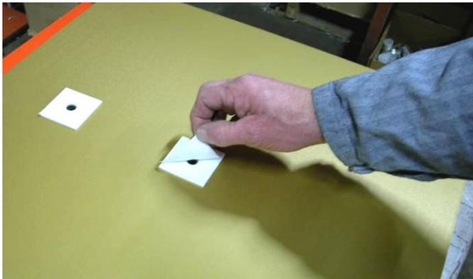
**STEP 4:** Remove the protective white sheet from the foam tape on the new element. Line up the inlet hole of the new air caster with the inlet hole on the mounting surface. **Holes must line up for proper operation, with the air inlet hole properly positioned.**
