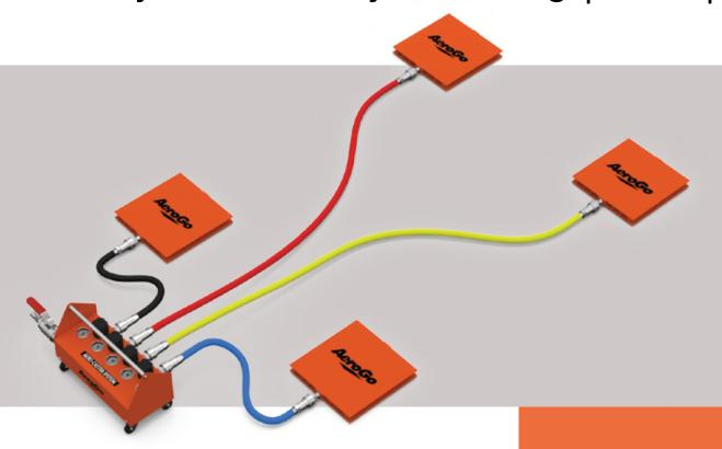
AeroGo® Gapmaster™ Air Caster Systems take advantage of the efficiency of air casters, a fluid film technology, which utilize compressed air to actually float heavy loads on a near-frictionless film of air.
