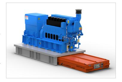
The AeroGo SILVERBACK Wheel Transfer Cart is engineered with precise movement proficiency through multiple steering modes. It can rotate within its own footprint, unlike forklifts or other conventional ride-on vehicles. The brake and acceleration function is designed to create the soft start/stop that prevents a multi-million-dollar product from "momentumsliding" off its perch on the cart. Upon delivery, a single operator easily maneuvers the transfer cart using a remote control.
