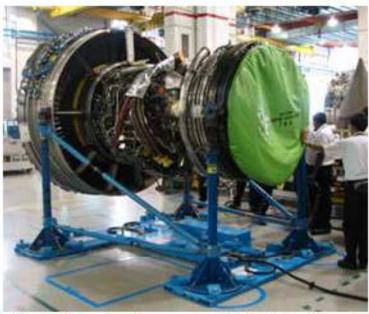
Safe tooling stand movement is facilitated by air bearings and power drive systems.
