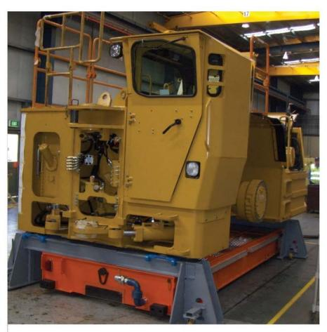
of force, only five to 25 pounds, is required to move a 5,000-pound load. Wheel casters may require up to 300 pounds of force for the same load. Because air casters are omnidirectional, very little force is required to change their direction. Industries that have relied on wheeled casters or rollers concede that directional change is time consuming, can gouge or tear floors, and is anything but flexible. Ramey agrees.
