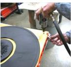
STEP 2: Remove the center bolt, center landing pad, and corner mounting bolts. On 27-inch models and larger, corner pads and a center pad are used. (NOTE: For Gapmaster models, no center-landing pad is used. Instead, cornerlanding pads are used.) Be sure to save all hardware.
