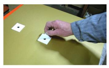
STEP 4: Remove the protective white sheet from the foam tape on the new element. Line up the inlet hole of the new air caster with the inlet hole on the mounting surface. Holes must line up for proper operation, with the air inlet hole properly positioned.
