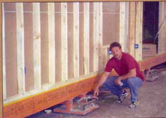
Jay Fink shows business end of AeroGo Air Casters which allow modular movement in any direction at Heritage Homes Modular Plant
