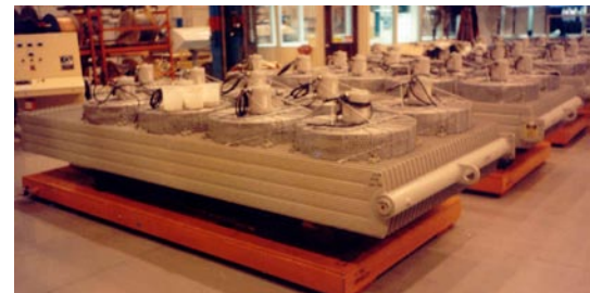
AeroGo Transporters ensure easy component movement through an assembly line. Line flow can be reconfigured on the fly, without downtime.
