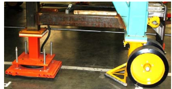
The High Lift Load Module uses standard shop air to lift and move scaffolding and tooling fixtures. Here, it provides additional lift height to a wheeled scaffold.
