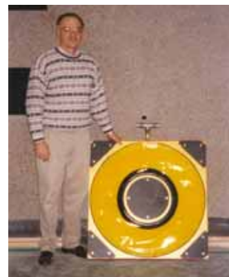
The 36-inch Urethane Heavy Duty Aero-Casters were chosen for their durability and expandable weight capacity.
