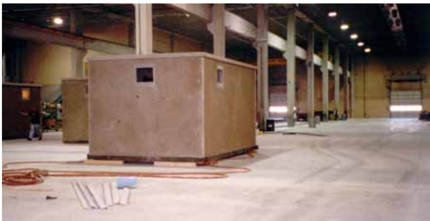
Assembly line flooring is easy to clean, polished concrete. Total travel distance is 150 yards/137meters. Once assembled, the buildings are loaded on to a flat bed truck at the loading dock with special pallet jacks.
