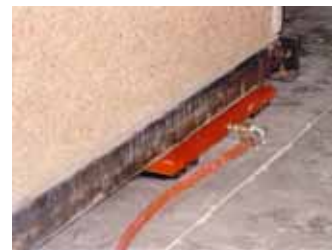
6K36UHDL Load Module Systems were inserted under each assembly to increase the production output and enhance production flexibility.
