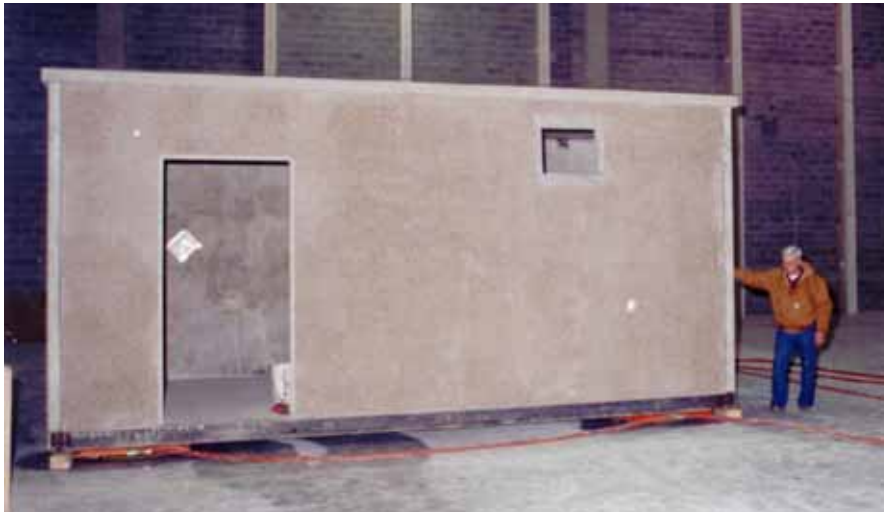
Microwave tower building manufactured on an Aero-Caster air bearing system with low ground clearance (3.5 inches/90 mm).
