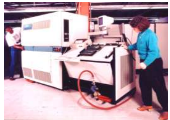
Versatile Aero-Planks can be used to move everything from machines to containers – anything up to 5000 tons.
