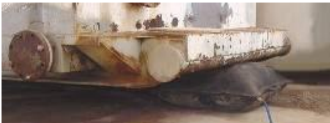
Aero-Jacks can be used to shift or lift the load in preparation for rigging.
