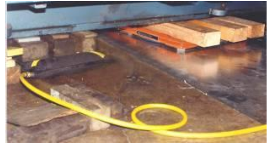
The thin profile of the deflated Aero-Jack makes it easy to insert under most loads. Here it is used on cribbing to increase lift height.
