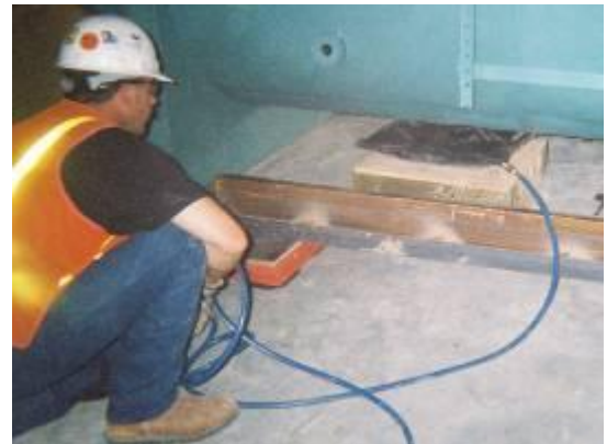
The thin profile of the deflated Aero-Jack makes it easy to insert under most loads. Here it is used on cribbing to increase lift height.
